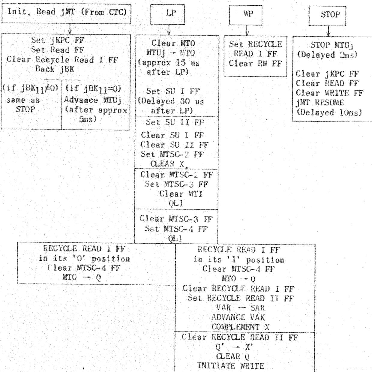
**Note:** Approximately 14ms after the pulse INITIATE READ jMT is received from CTC, a line pulse (LP) is generated by MTUj. Approximately 15us after the LP is produced, the transmission MTUj → MTO occurs. MTUj generates successive LP's at the rate of 4 1/2 kc. Along with each 18th LP, LK generates a word pulse (WP). Along with each 32nd WP, WK generates a block pulse (BP) which subtracts one count from the preset block count (BK). When BK = 0, the BP becomes a STOP pulse.
