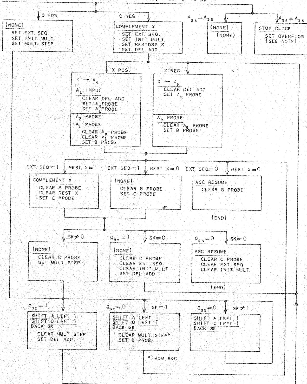
NOTE: SETTING THE OVERFLOW FLIP-FLOP PRODUCES AN A FAULT. CLEARING THE A FAULT CLEARS THE OVERFLOW FLIP-FLOP AND ALLOWS THE ASC MULTIPLY SEQUENCE TO PROCEED.
