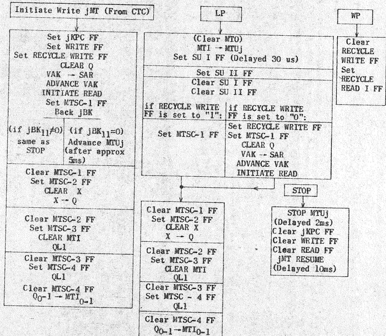
Note: Approximately 14ms after the pulse INITIATE WRITE jMT is received from CTC, a line pulse (LP) is generated by MTUj. MTUj generates successive LP's at the rate of 4 1/2 kc. Along with each 18th LP, LK generates a word pulse (WP). Along with each 32nd WP, WK generates a block pulse (BP) which subtracts one count from the preset block count (BK). When BK=0, the BP becomes a STOP pulse. (As before each gated LP clears MTO, however this is of no significance in the MT Writing operation.)
