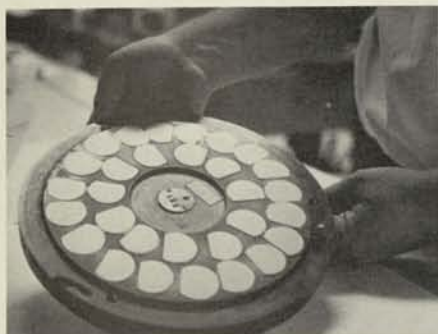
1. As mentioned previously, the wafers are waxed down on grinding discs before being sent to Lapping or Polishing.
