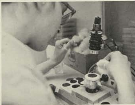
4. After polishing and demounting from the discs, Rita Ramirez carefully cleans each wafer with alcohol-soaked cotton. Depending upon their classification, the slices are now ready for either Oxidation or Epitaxial Growth.
