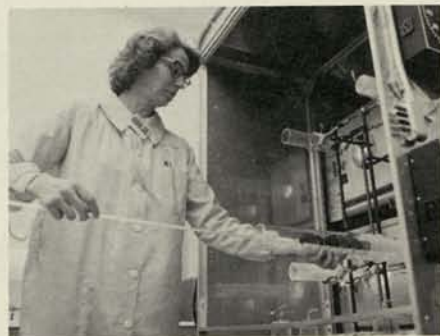
5. If sent to Oxidation, quartz boats full of wafers are placed in an oxidation furnace, as performed by Gloria Blondin. At a given temperature, silicon dioxide is transformed into an oxide layer on the polished surface of each silicon wafer.
