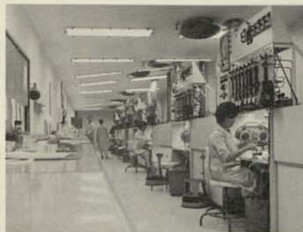
6. If destined for the Epitaxial Growth area, large reactors utilize distilled silicon tetrachloride to grow another layer of silicon on the polished slices.
