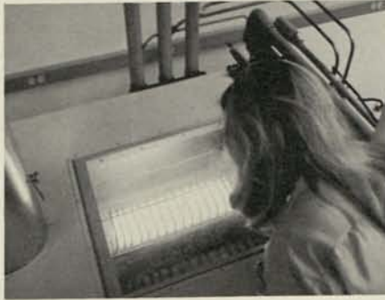
7. Donna Smith peers down at wafers in an epitaxial reactor. The original "substrates" (wafers) possess high conductivity, while the silicon layer that is grown during the process, has low conductivity.
