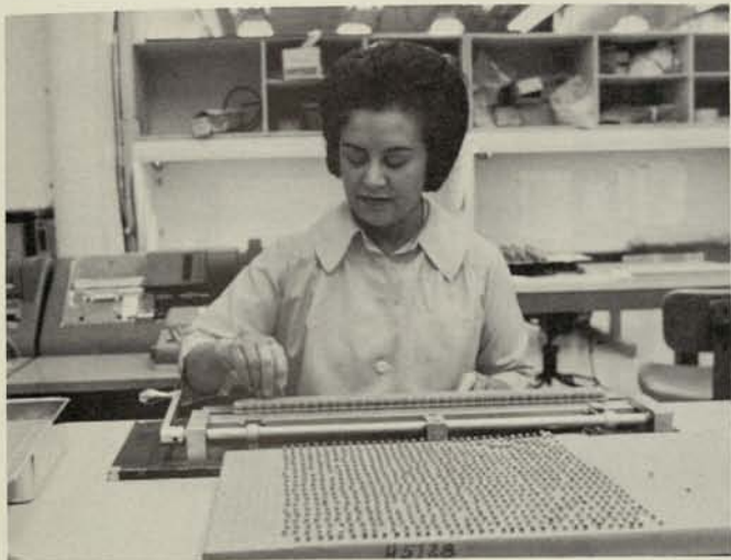
2. Carol Lujan loads transistors in sockets for stabilization burn-in. The units are operated at a uniform power voltage specified by Motorola.
