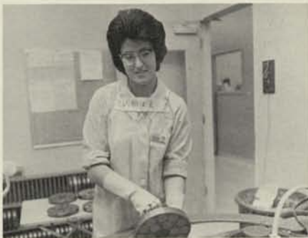
2. In Lapping, Virginia Reyes places the discs on a revolving grinder table. The difference between the Lapping and Polishing processes is merely the grid (or abrasive). Here, a 12.5 micron aluminum oxide paste is used for 20 minutes on the slices.
