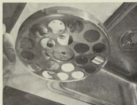
3. Dorothy Brown's face is reflected in wafers which have been polished. One micron diamond paste has been used as the abrasive agent.
