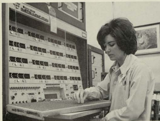
3. According to a multitude of Motorola parameters, the devices are tested on Instrumentation's 500B system by Karen Valdespino. The tests performed are then punched on EDP cards.
