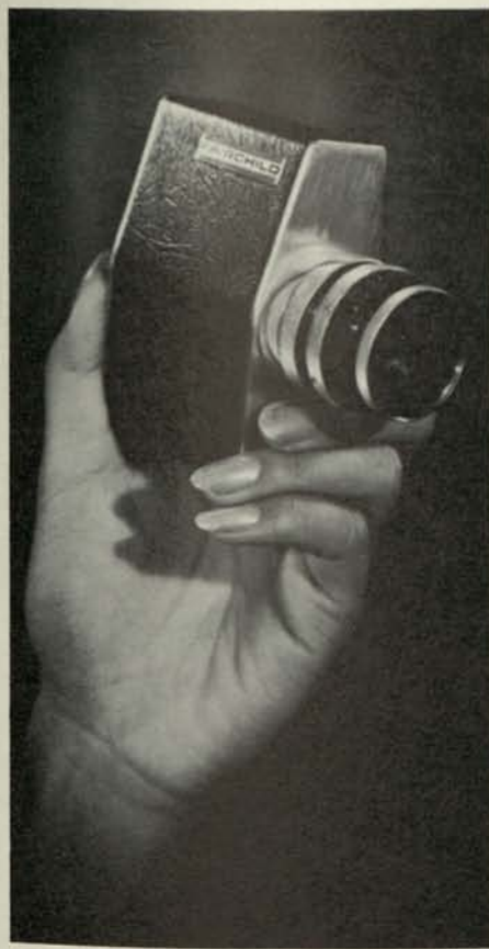
The Fairchild Space & Defense solid-state television camera measures 3\frac{1}{2} \times 1\frac{1}{2} \times 2\frac{1}{4} inches and weighs 6 ounces.
