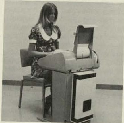
The new teletypewriter terminal buffer (TTB) may be mounted on the back (left) or side (right) of the TTY with no cutting or drilling. The TTB accumulates messages generated on the teletypewriter for later transmission at high speed.
