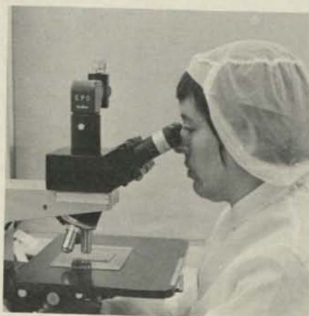
Win Williams, Q.C. operator, inspecting an emulsion working plate.
