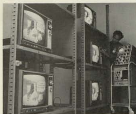
Tony Brooks checks out TV receivers in CARE (Component Application and Reliability Evaluation) facility.
