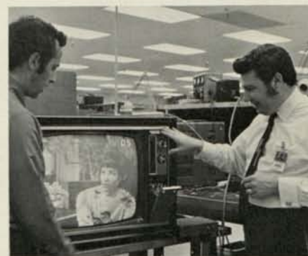
Tony Brooks and Halfon Hamaoui, Consumer Applications, demonstrate an on-screen TV channel number display.
