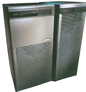
AlphaServer 8000 systems support up to 14 symmetric multiprocessors, DIGITAL UNIX TruClusters, 28 gigabytes of memory and 39 terabytes of storage to provide better-than-mainframe and supercomputer performance. Business-critical applications include data warehousing, high-performance technical computing, sophisticated telecommunications applications and large-scale database management.
