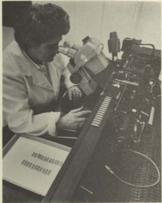
Semiconductor mounting and several other operations are performed under clean room conditions in the manufacture of the hybrid integrated circuits for the FLIP CHIP Modules
