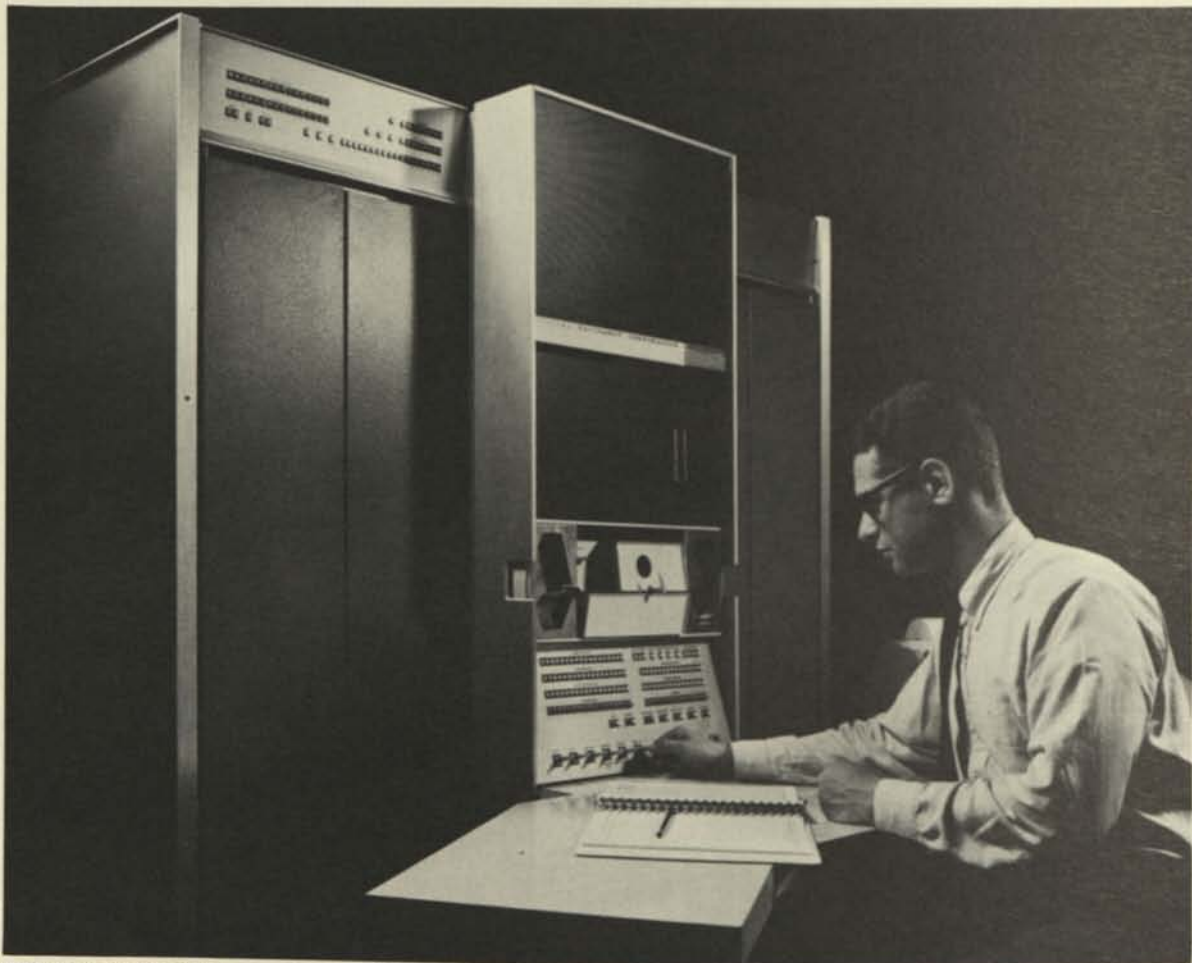
PDP-7 computer, which was developed from our earlier PDP-4 has FLIP CHIP Modules that make it more than four times as fast and permit a price reduction of more than 20 per cent
