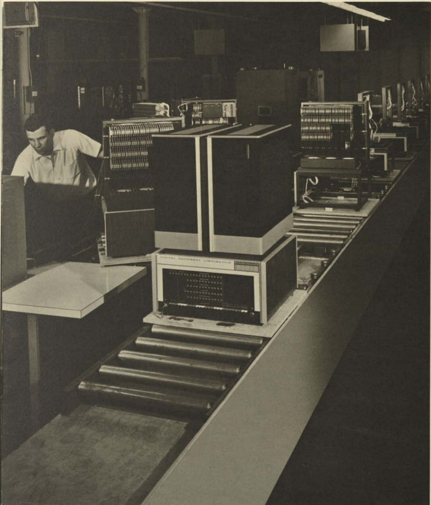
The significance of the assembly line now being developed is that it centralizes all steps in building and checking a PDP-8, including the use of computers to test components before assembly
