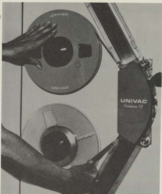
Figure 4-8. Tape Threaded Over Lower Vacuum Column
