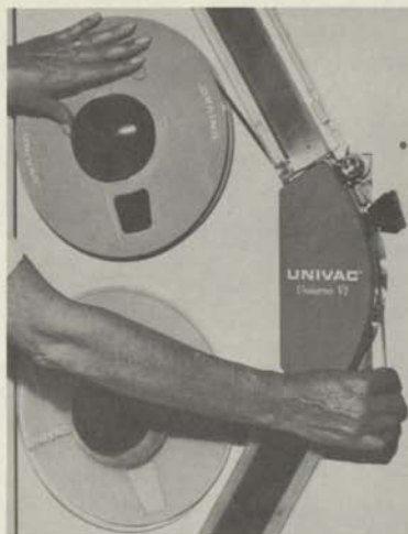
Figure 4-7. Tape Threaded Down Over Read/Write Head
