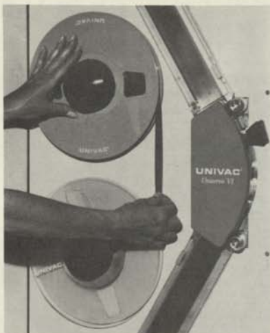
Figure 4-5. Tape Reel Mounted on Supply Reel Hub
