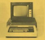
be supplied as an option. Its interface conforms to the CCITT V24 standard. The console is to be connected to Micral through asynchronous coupler M1403.
