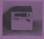
The magnetic cassette unit represents a low-cost storage facility for small files when a magnetic tape unit is not required
