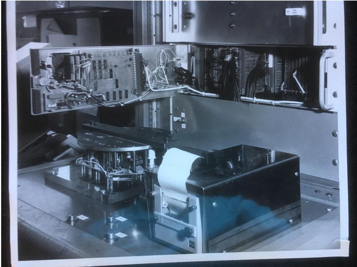
Source Paul Russo: CLOSE-UP OF TV FACTORY MICROPROCESSOR-BASED AUTOMATIC CONVERGENCE ADJUSTMENT. BLOOMINGTONTN INDIANA RCA TV FACTORY.
