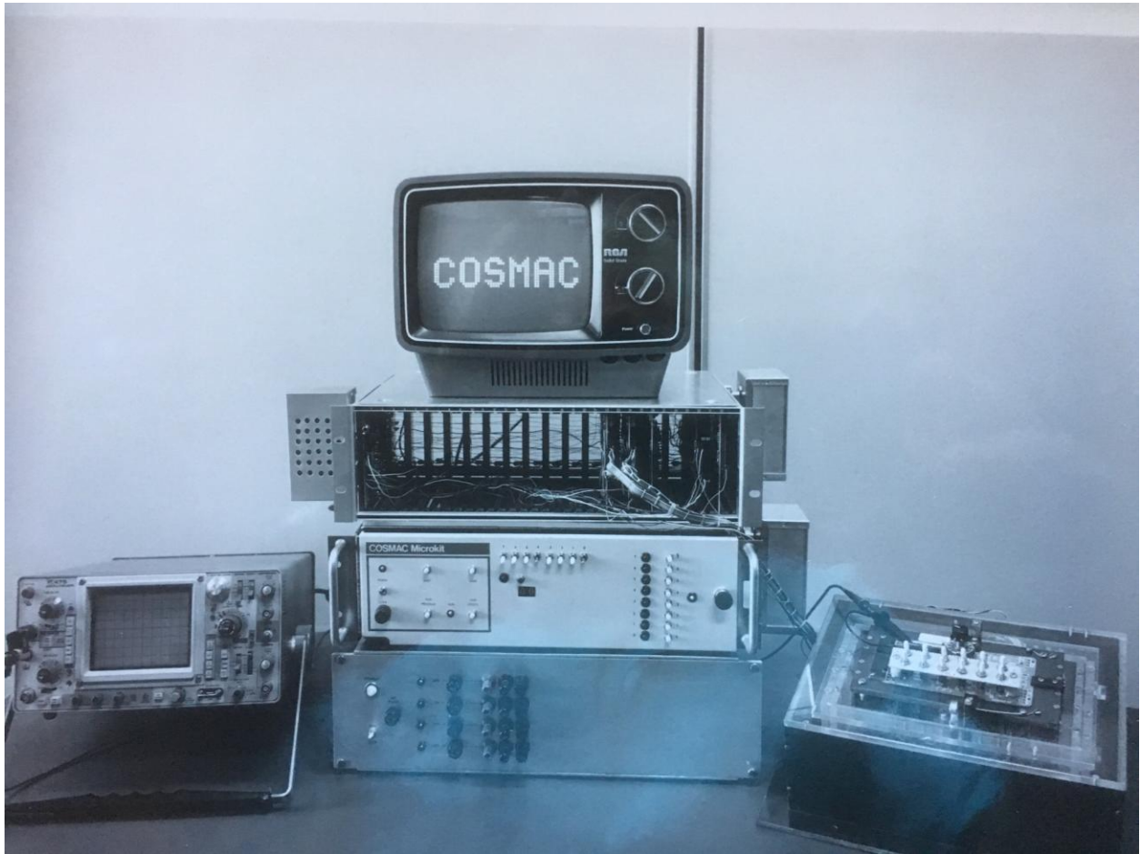
Source Paul Russo: FIRST TWO-COSMAC SYSTEM MULTI-PROCESSOR SYSTEM: TWO COSMAC 1802-BASED SYSTEMS TALKING TO EACH OTHER TO ACCELERATE COMPUTATION.
