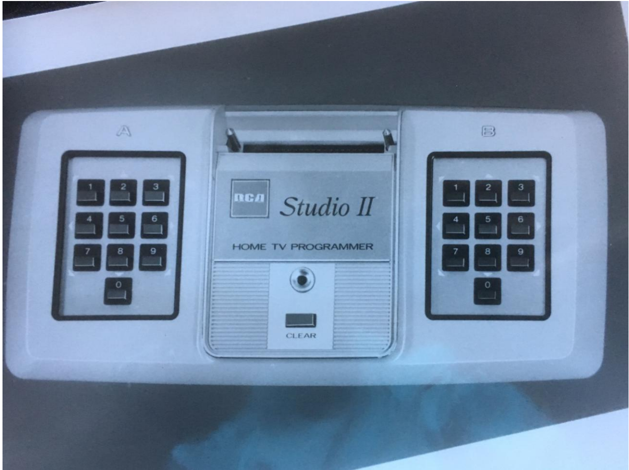
Source Paul Russo: STUDIO II CONSOLE: WORLD'S FIRST VIDEO GAME CONSOLE WITH PLUG-IN ROM-BASED CARTRIDGES FOR GAMES. BLACK AND WHITE, 64X32 DOTS DISPLAY.
