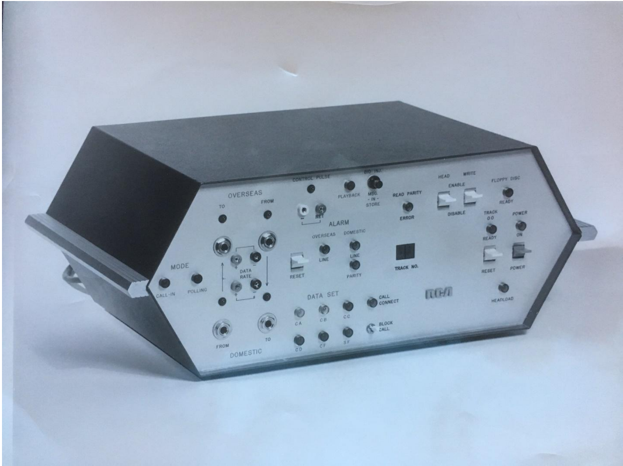
Source Paul Russo: GLOBAL COMMUNICATIONS 1ST MICROPROCESSOR CONTROLLED BIT RATE AND FORMAT CONVERTER TO REPLACE PAPER TAPE SOLUTIONS CLOSE-UP OF SYSTEM BOX WITH FLOPPY DISC CONTROLLER.
