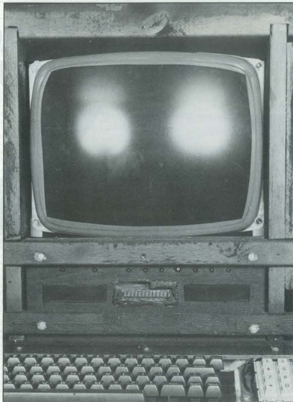
Display panel with smoked plastic cover removed.
