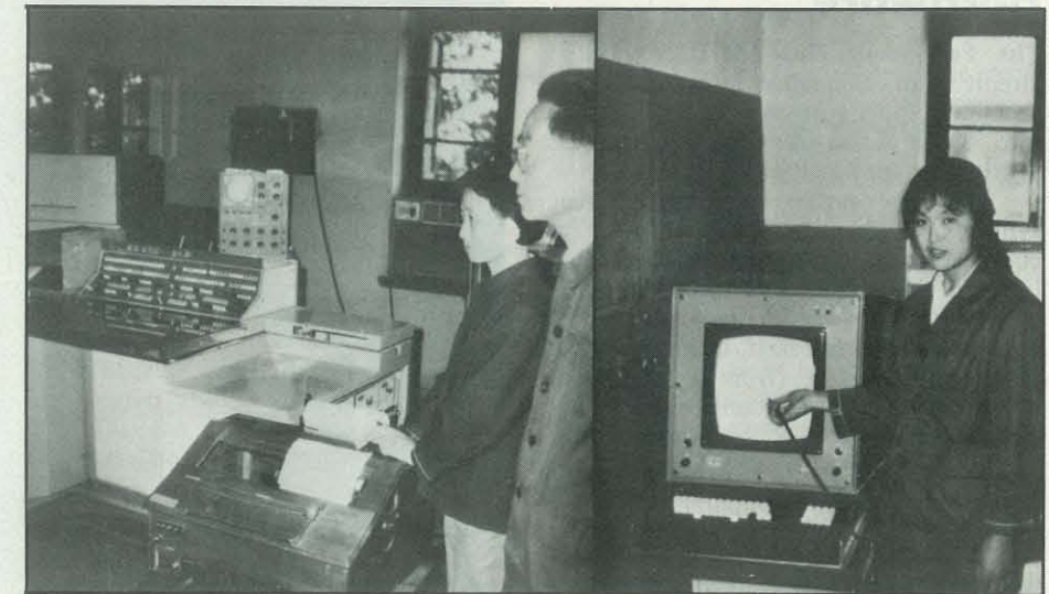
A Chinese 16-bit minicomputer (left). A Chinese designed and built light pen graphics terminal (right).
