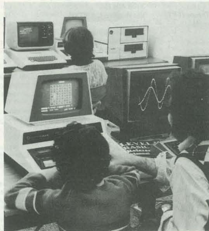
Fifteen computers, each doing its own thing, can be connected to a central disk file via the Cluster/One system.
