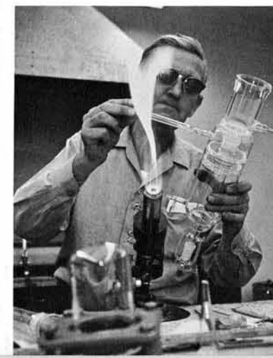
Tooling so precise it is done under magnification—hand-blown laboratory glassware—custom-machined copper fittings: typical of work from the experimental machine shop.
