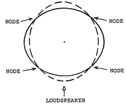
FIGURE 2. VIBRATION PATTERN OF GOBLET RIM AS SEEN FROM ABOVE
