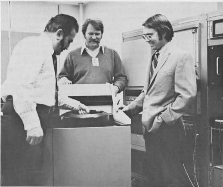
Al Hasler places a Memorex Disc Pack on the new 3675 Disc Module during a thermal expansion test which analyses temperature effects on the drive's operation, while Ron Higgins and Robert Tempero look on. Dave Reece (not pictured), has recently been promoted to Mechanical Engineer II and is now a member of this team.
