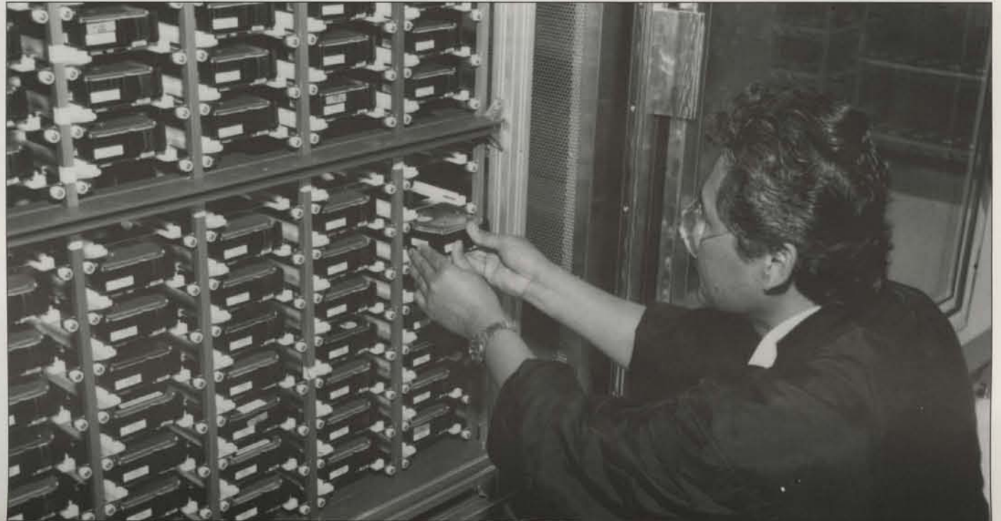
Targeting worldwide certification... Milpitas is ISO9001 certified for design, build, inspect and test. Here, Crispin Amores loads a Grand Prix drive into a Drive System Test chamber.
