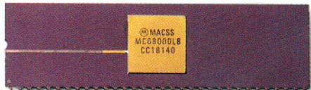
Macintosh's 32-bit microprocessor.
