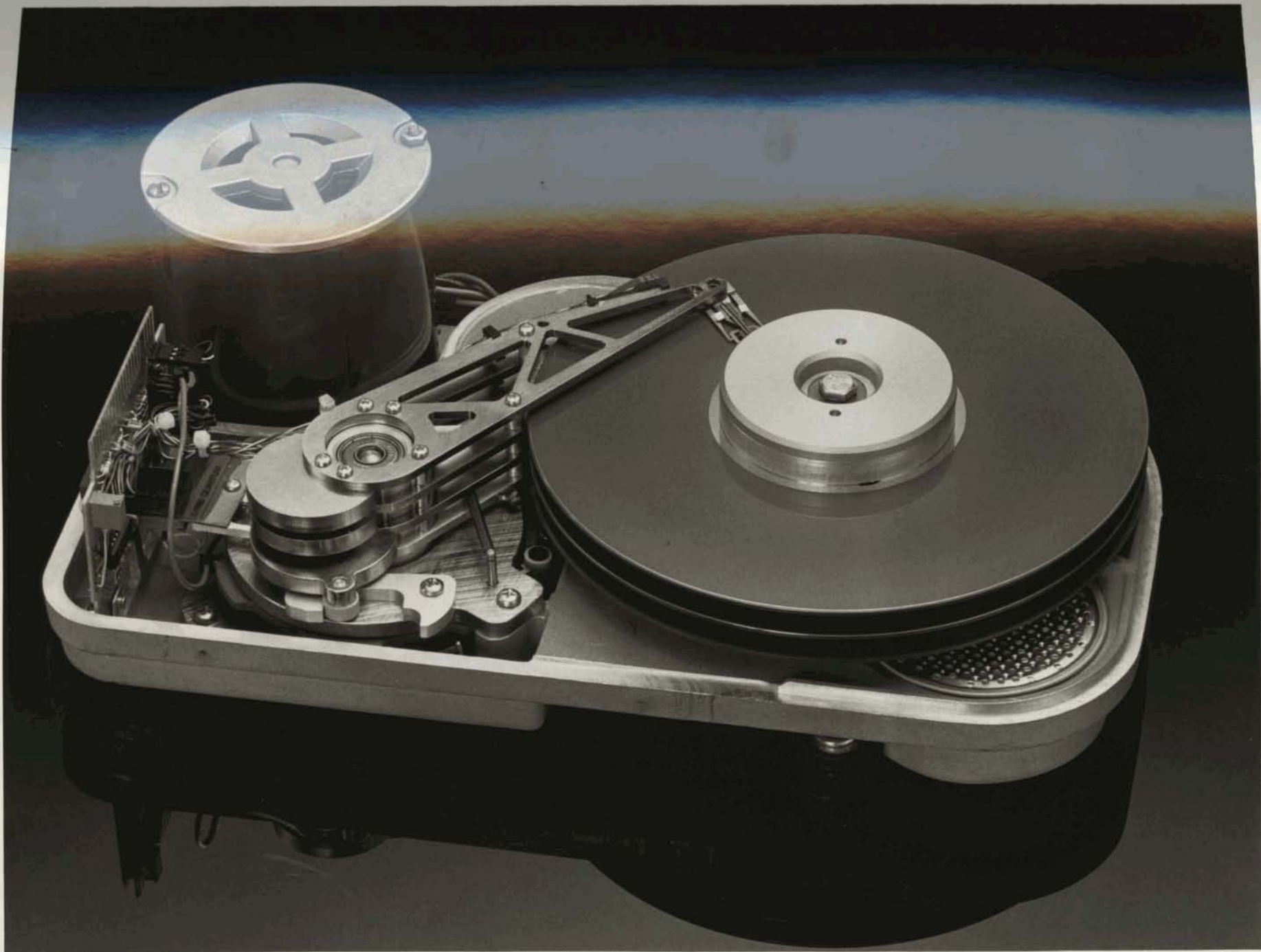
Internal design of 30 MByte Q2000 8-inch fixed disk drive (bubble removed) from Quantum Corp.
