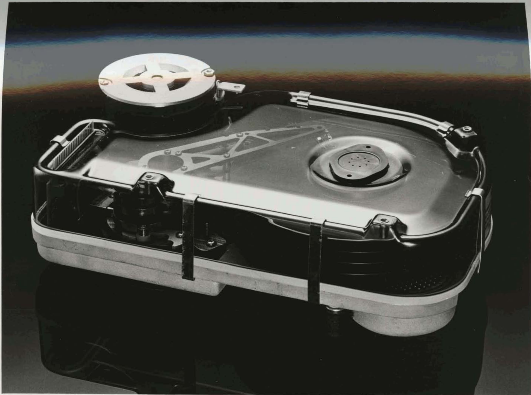
Q2040 40-megabyte 8-inch fixed disk drive from Quantum Corp.
