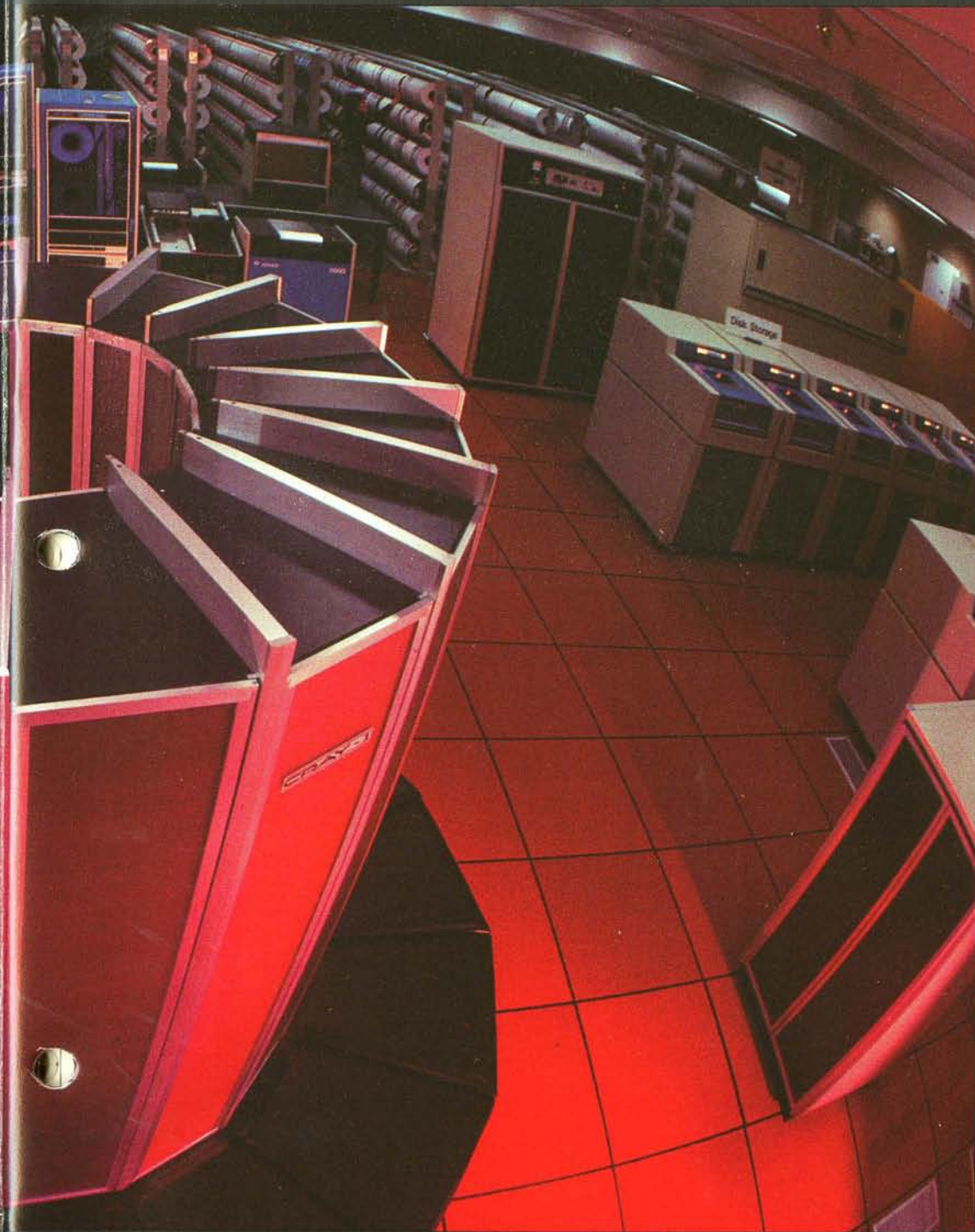
The Cray I computer, shown here at the National Center for Atmospheric Research in Colorado, is the world's most powerful information processing machine. The CPU (foreground) of each Cray computer contains 250,000 dual subnanosecond ECL gates and 65,000 1K ECL RAMs, all supplied by Fairchild.
