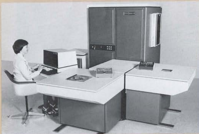
The Sentry VII computer-controlled semiconductor test system, introduced in September, provides reliable and efficient testing of microprocessors, high-density memories and other circuits.
