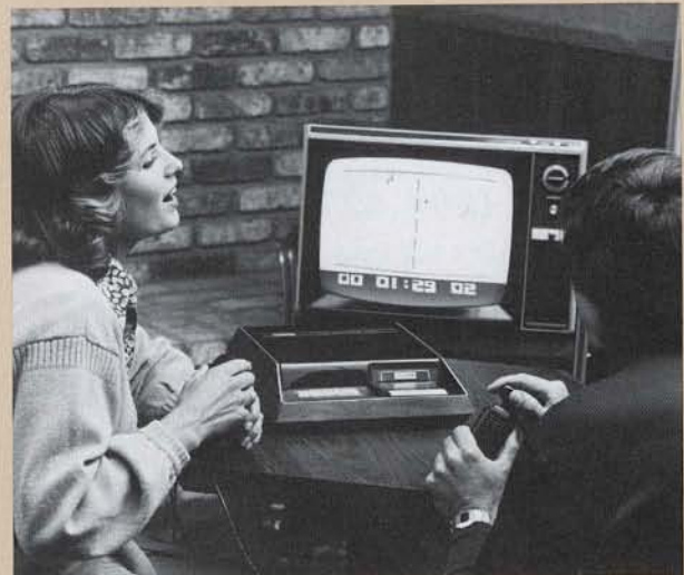
The Video Entertainment System, first shown at the June Consumer Electronics Show, uses replaceable cartridges and incorporates Fairchild's F8 microprocessor.
