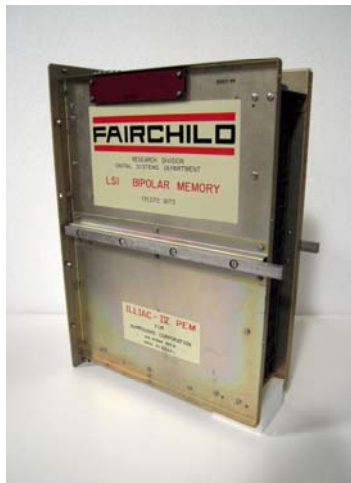
Iliac IV Processor Element Memory system that holds the board on display
