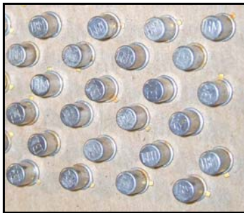
Section of Cardboard Box Packaging for 200 Type 154 Transistors. Overall Box Size = 10 3/4" X 3 1/2" X 2". Individual Transistors Not Labeled, and Not Packaged Individually.
