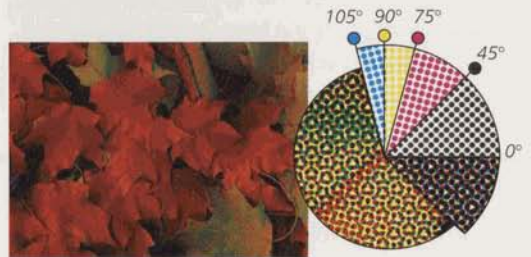
Halftone screens with process inks at different screen angles; correctly registered dots form rosettes
