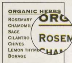
Process colors in small type and fine elements are more likely to show misregistration.
