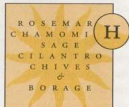
Small spot-colored text set to overprint, misregistered.
