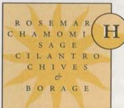
Small spot-colored text set to knock out, misregistered.
