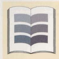
Color shifts can occur when crossovers print on different forms.
