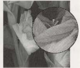
Image resolution: 300 ppi Output resolution: 2400 dpi
