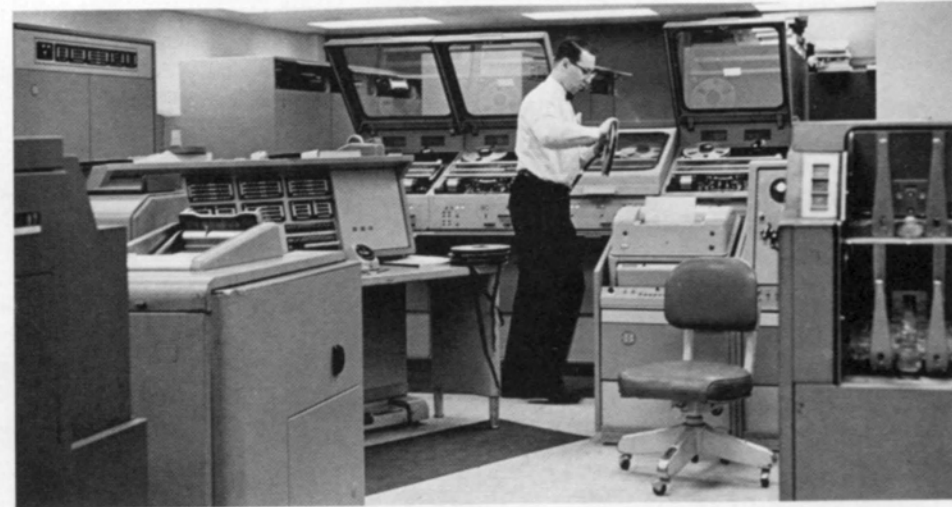
FIRST OF THE computers installed at Case Tech was the IBM 650 (top, background). Frederick Way III (center, left) was the first assistant director and Dr. Raymond J. Nelson, the first director of the Computing Center. Next were the Burroughs 220 (right) with Albert E. Misek '53 shown with a reel of tape.
