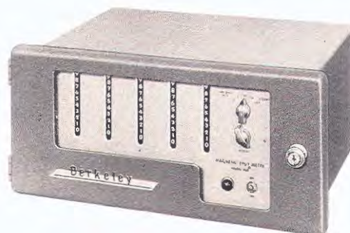
Model 7650 Long Life Magnetic EPUT® Meter performs the same function as models described above. Uses Berkeley FERRISTORS* in all critical circuits to assure continuous-duty reliability. Ideally suited to industrial test applications such as jet and piston-engine test cells, etc. Has digital "count-down" time base for precise gating; no adjustment of time base required.
