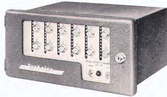
Series 5840 long-life magnetic dual preset counter features FERRISTOR* circuitry; 4-digit, $1115.00; 5-digit, $1200.00; 6-digit, $1295.00.
