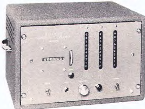
The Berkeley Industrial Counter, Model 5010 (10 KC), is a high-speed electronic counting instrument designed to fill general counting needs, where speed requirements are greatly in excess of those possible with mechanical counters.
