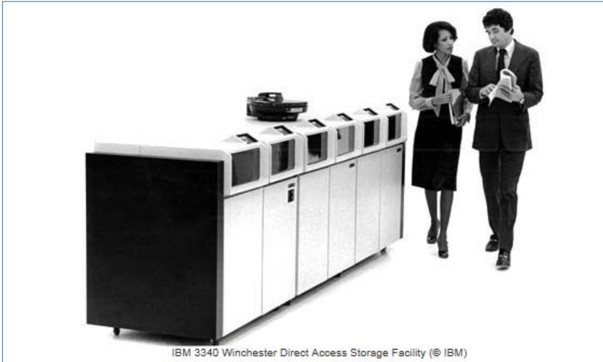
View of IBM 3340 drive, with IBM 3348 Data Module pictured on top. System was announced together with IBM 370 model 115 processor in 2, 4 or 8 unit configuration, with 280 MB total capacity with 35 MB IBM 3348 Data Module.
