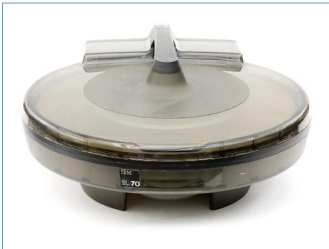
IBM 3348 Data Module for the IBM 3340 drive, containing either two or four 14-inch disks with capacities of 35 or 70 MB. The module had a spindle with bearings, head carriage, and a head-arm assembly with two low mass flying head per surface (Reference 4-1).
