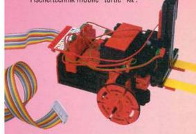
Start by building the turtle, following the simple illustrated instructions. Attach it to the interface and connect that to the computer. Load the special Logo files and you are ready to control the turtle from the computer by typing commands, just as you would to move the on-screen turtle!
