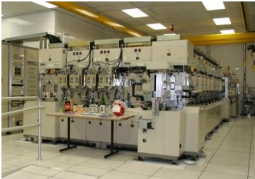
Left, a photograph of modern Anelva 3040 sputter system at the time of installation ceremony at Komag and at right, an Intevac Lean System (courtesy of Intevac Inc.). (Figure 12-3)
