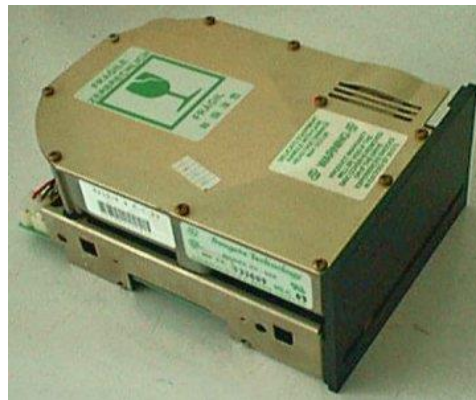
Seagate ST-506 Drive, designed to fit into 5.25-inch floppy bay of IBM PC. Drive had 5MB capacity on 2 oxide disks.
