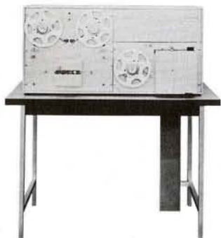
PAPER TAPE CART with 300 cps Reader, 60 cps Punch, and Spooler
