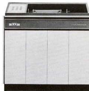
LINE PRINTER, 600 lines/min., 132 characters/line, 64 printable characters.
