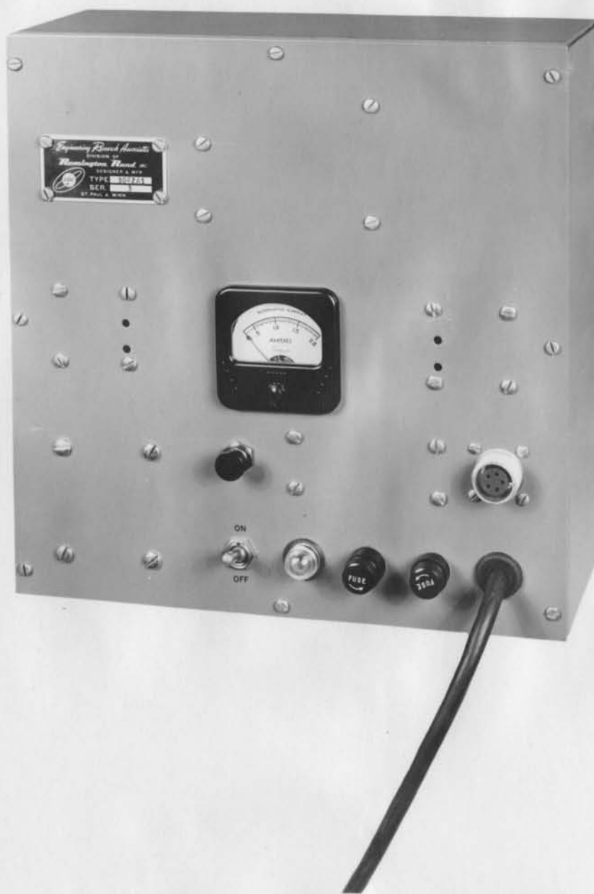
Plate 5-23. Magnetic Drum Erase Equipment (28500 Unit)
