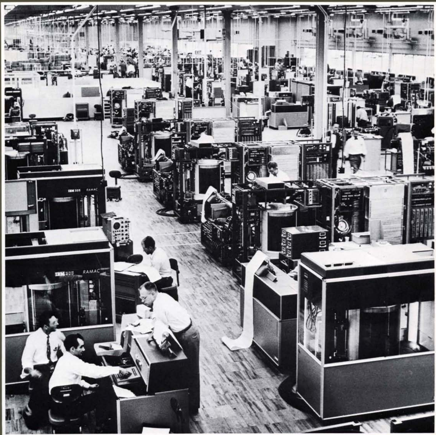
Development of the 350 RAMAC file at San Jose led to the company's decision to build its first computer manufacturing plant in California. Above, engineers test units of the 350 RAMAC System before customer shipment from the new facility in 1957.
