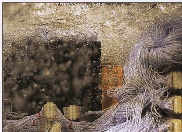
The CRAY-3 modules are continually bathed in a precisely controlled flow of a clear, inert fluorocarbon. The presence of this liquid can only be visually detected by an occasional bubble, or when the tank is being filled.
