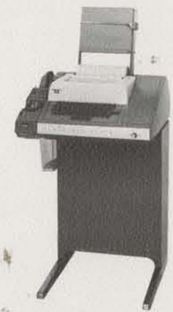
TELEPRINTER Keyboard, punch, read, print 10 char/sec ASCII character set
