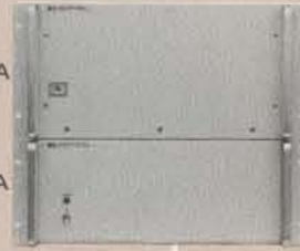
DISC MEMORY (2116B, 2115A only) 32 tracks, head-per-track 2720 addressable sectors 64 words/sector 174,080 16-bit words (64-track disc also available)
