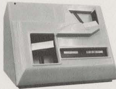
CARD READER 12-bit parallel column, 80-column cards 1000 cards/min
