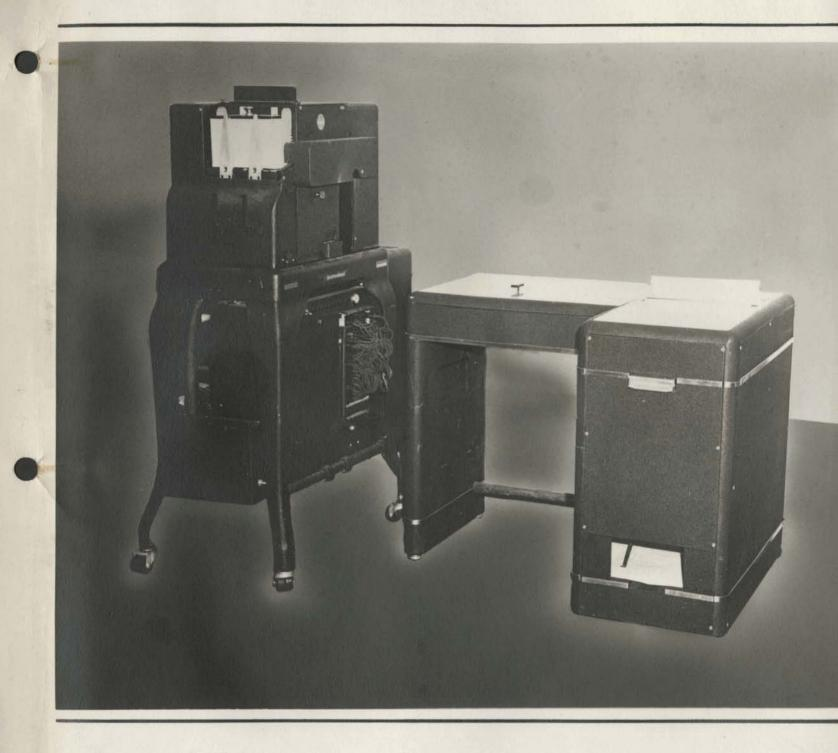
This machine consists of a combination mark sensing reading unit and card punch which permits the automatic preparation of I.B.M. cards from marked original documents. It was developed by Mr. R. B. Johnson from an original suggestion by Mr. Watson.
